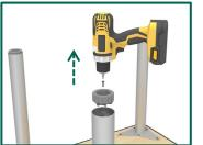
Remove the screw located at the center of the glide. Once free remove the glide. Repeat for all 4 legs.
